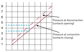
\* EXAMPLE: Pressure at connection 3,5 bar Pressure at disconnection 4,5 bar
